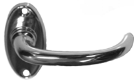
18.931F SET: Passage Classic Latch with oval escutcheon and ships lever + strike plate Lever handle classic, big #18.956 + oval escutcheon #18.931; half size latch #14.220 Lever handle 107 x 42 mm; Escutcheon rose, oval: 82 x 38 mm Latch: see page 1-4-L
